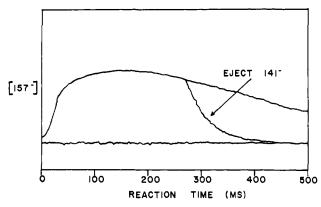
Figure 2. Ion cyclotron double-resonance ejection time plot for m/z 157 with ejection of m/z 141 from m-fluoronitrobenzene. The rapid decay of m/z 157 indicates that electron transfer between the two nitrobenzenes is rapid.
