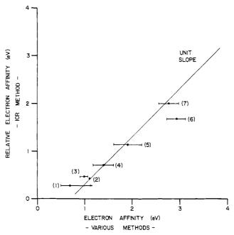
Figure 4. Comparison of relative electron affinities determined by the pulsed ICR equilibrium method with absolute EA's measured by various other methods: (1) nitrobenzene;<sup>27</sup> (2) SO<sub>2</sub>;<sup>28</sup> (3) phthalic anhydride;<sup>29</sup> (4) maleic anhydride;<sup>30</sup> (5) benzoquinone;<sup>31</sup> (6) fluoranil;<sup>32</sup> (7) chloranil;<sup>32</sup> (7)
